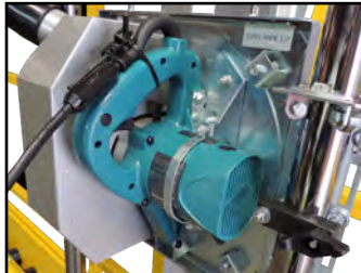
Makita Saw on Spinning Insert
