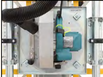
Makita Saw on Spinning Insert + Dust Collection
