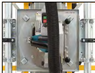
Makita Saw on Spinning Insert + Dust Collection
