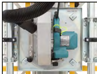
Makita Saw on Spinning Insert + Dust Collection
