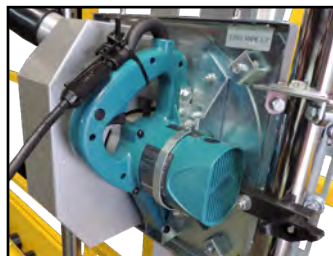
10" Saw on Spinning Insert + Dust Collection
