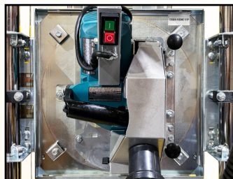
Makita Saw on Spinning Insert + Dust Collection
