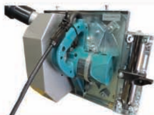
10" Saw on a Spinning Insert w/Dust Collection
