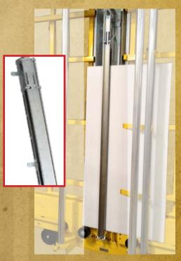
Giving you that extra hand to hold the material in place, so that you don't have to! It is especially useful when cutting long, narrow pieces on the material rollers, or small pieces on the mid fence. Magnets are used to hold it open. 48" capability.
