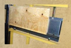
Allows for easy, waist-high cuts instead of cutting smaller pieces down by your ankles. Lip is removed for cutting full sheets. All metal construction, won't warp, swell, or de-laminate. Removable lip holds small material in place waist-high.
