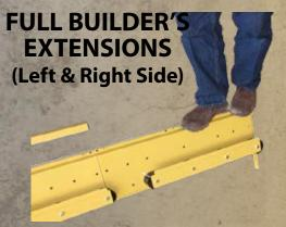
Each extension is 28" long. Used to extend the wheel base of the machine to provide added material support when feeding or exiting materials during a rip-cut. Extensions are easily added or removed with self-aligning bolts. Perfect for taking to the job site with a compact machine.
